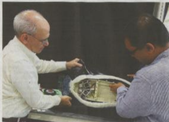
A GOOD FIT Prof. Nicholas Patrikakis, left, displaying the inside of an underwater robot for collecting data on ocean algae. Students don't have to go far; test beds are right off the coast.
